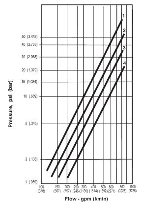
Curve 1 Model 60427CF\*6H nozzle with 100-mesh screen, HECV and 2½-inch inlet
